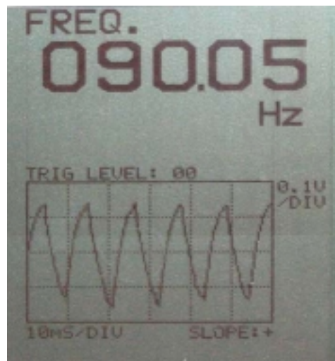
Fig. 7 The second controller's output and update cycle frequency, after a clock fix
