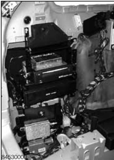
The left side storage compartment contains the NAV computer when installed and the telephone transceiver and CD changer.
