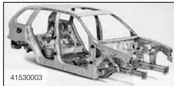
In addition to the cross bracing on the front suspension/engine carrier, an additional panel is installed between the bulkhead and transmission tunnel.
