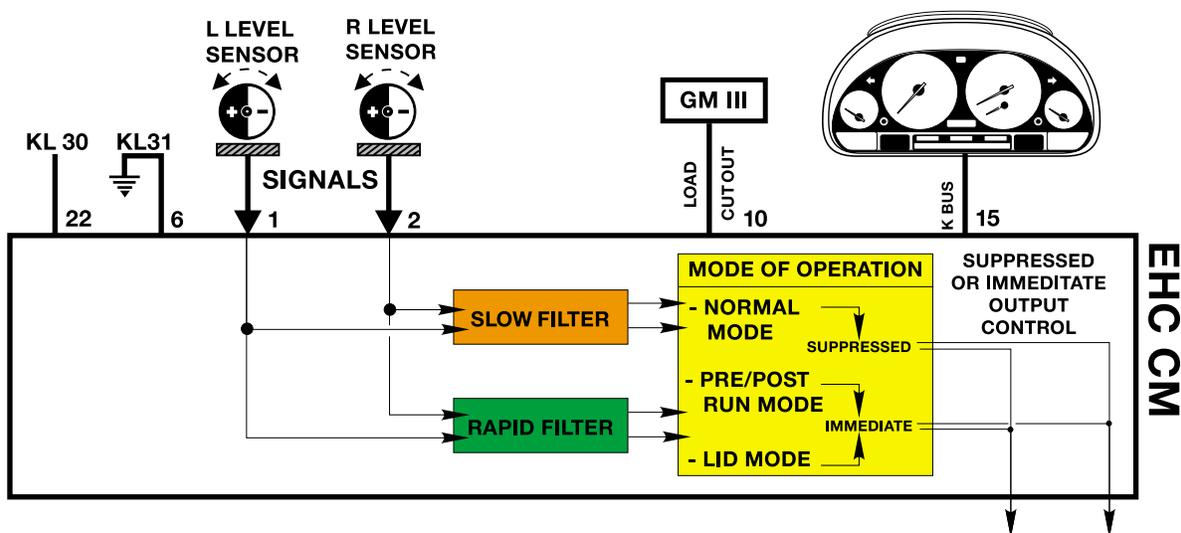
The rapid filter is used during the pre-run and tailgate (LID) modes to ensure that the suspension is adjusted quickly while the vehicle is being loaded or checked prior to operation.
