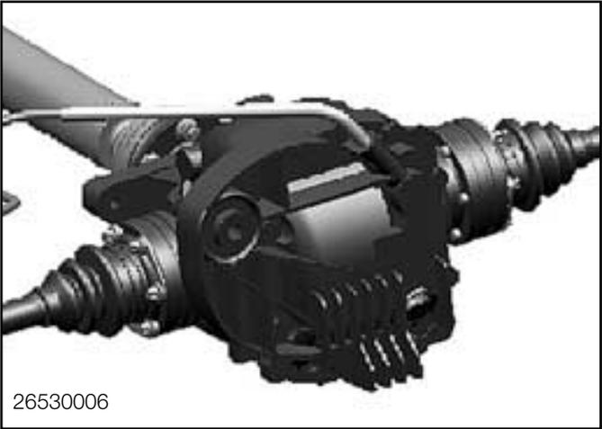
The front differential is the VAG 174 unit with a ratio of 3.64 : 1.
