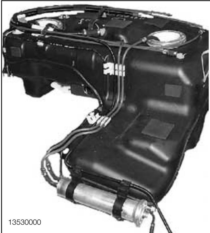
The fuel filter/pressure regulator is mounted in front of the tank along with the charcoal canister. The components are covered by a plastic plate to protect them when driving off-road.
