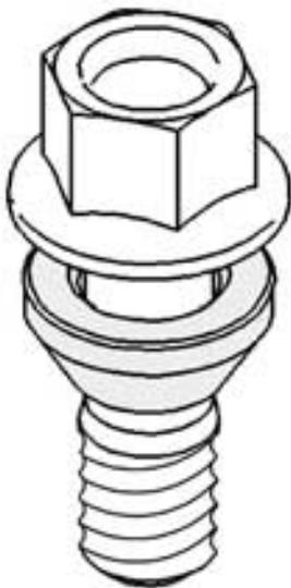
The X5 uses a two piece lug bolt that incorporates a spacer washer and features anti-corrosion coating. The tightening torque on the lug bolts is 130Nm +/- 10Nm. Advantages of using the spacer washer include:
