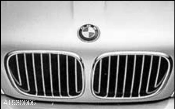
The grilles are integrated into the hood with the secondary hood latch springing out from the grille when the hood is opened.
