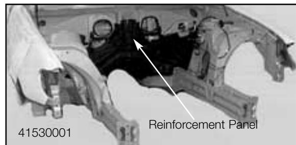
The floor pan of the X5 is reinforced with additional ribbing and cross braces to increase the lateral rigidity. A continuous seat cross brace is connected to the floor pan and side sill for reinforcement.
