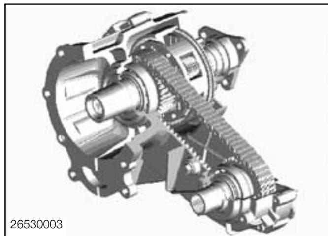
A torque split of 68% rear/ 32% front is provided through the gearing of the planetary set.
