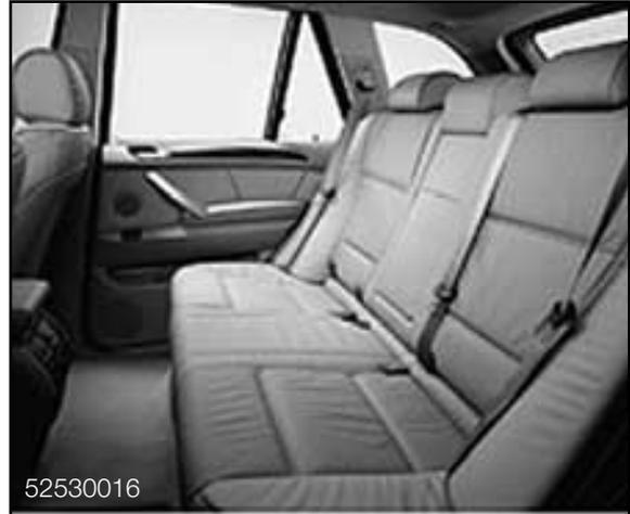
The rear seats have a 60/40 split with the fold down center arm rest on the left seat back. The center arm rest also includes the optional folding ski bag.
