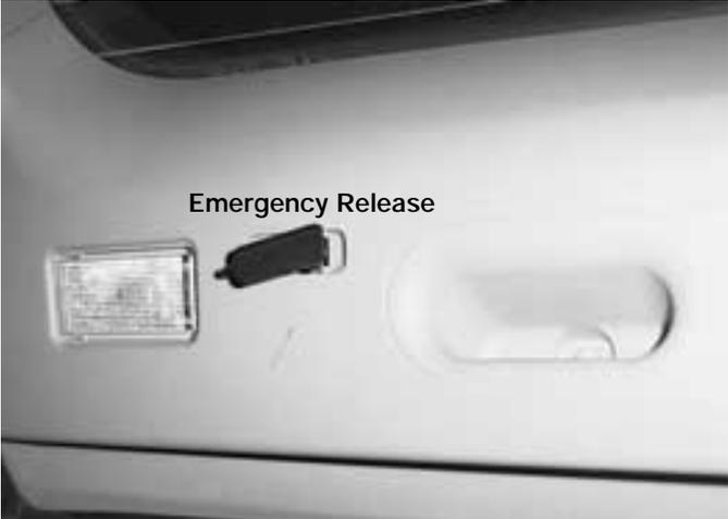
The lower tailgate emergency release is accessed by removing the trim cover on the tailgate section. With the gate closed, only the top section will be able to be loosened. The mechanical release is actuated by inserting a small screwdriver into the opening and pressing the latch to the left.
