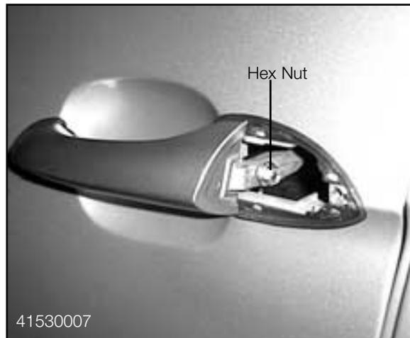
The handle is then removed by pulling it out and down to release it from the latch. The handle is turned down to the left to release it from the door latch assembly.
