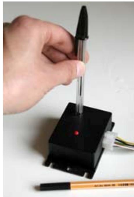
The LED should now either start to output longer, 0.25–0.75 s flashes or blip, just once, every few seconds. If it continues to output trains of 50 ms blips, the number of coding blips didn't match. Repeat steps 3–5 until the LED starts to blip once or flash for longer. The controller is now ready
