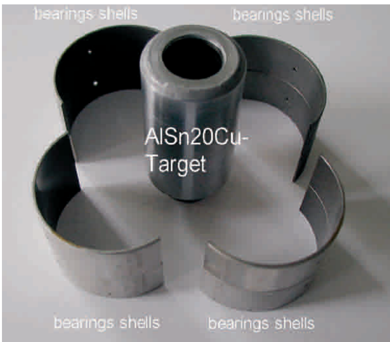
Fig. 5: Half bearing/target arrangement (multi-chamber unit, type B)
