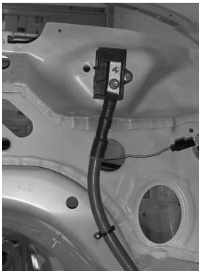
Cable Routing on Firewall
