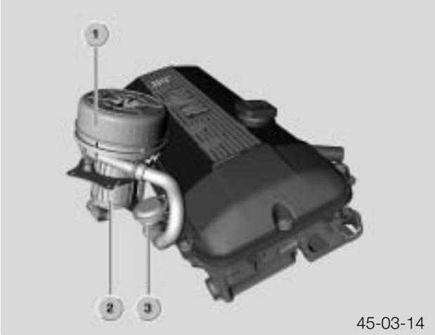
The electrically driven secondary air pump is mounted to the body in the engine compartment (in the area of the right-hand strut tower). To draw in secondary air, the SLP has an integrated air filter element. The air filter element is maintenance-free during the service life of the vehicle.
