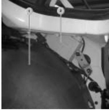
1. Wheel Arch Trim 2. PDC Control Unit
