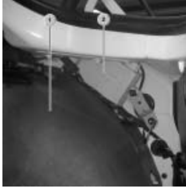
1. Wheel Arch Trim 2. PDC Control Unit
