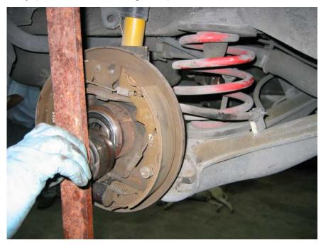
After your bearings are press in, you can press in the hubs.
