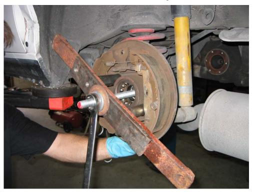
Or, you can use a puller. This one was a cheap-o model and broke on us.
