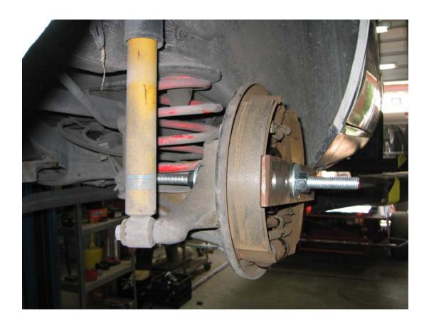
Next, all you do is **LIGHTLY** tap your axles back in. This is where you want to make sure those splines match very easily. Then, bolt them back up to the differential, put the brake drum (or disc and caliper) back on, replace the wheels and you're done!
