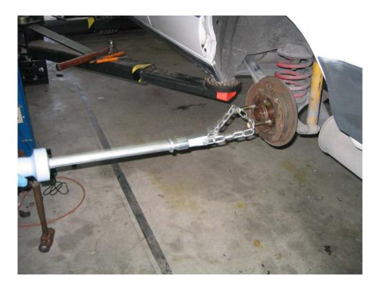
Once the hubs were out, we knocked out the inner race from the wheel hub.
