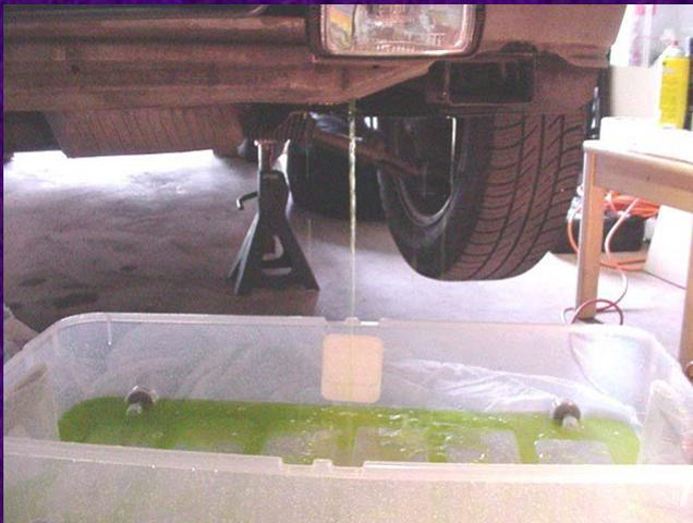
Drain the coolant from the system, and make sure you also drain the engine block by unscrewing the 19mm drain plug by the exhaust manifold.
