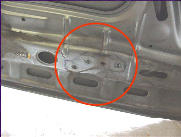
Before removing the hood, trace the hinges with a Sharpie or other pen so alignment is easy when you put the hood back on.
