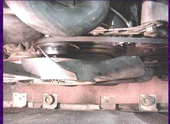
Reattach the fan & clutch. Again, I used a strap wrench to hold the pulley steady and the Channel-Locks to tighten the fan nut to the water pump shaft. Remember, it goes on COUNTER-CLOCKWISE..
