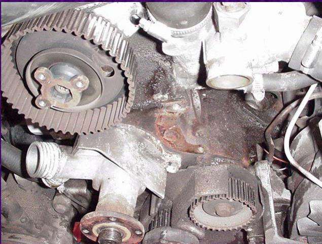
Remove the tensioner gently, making sure that the spring and adjustment pin don't fly out!
