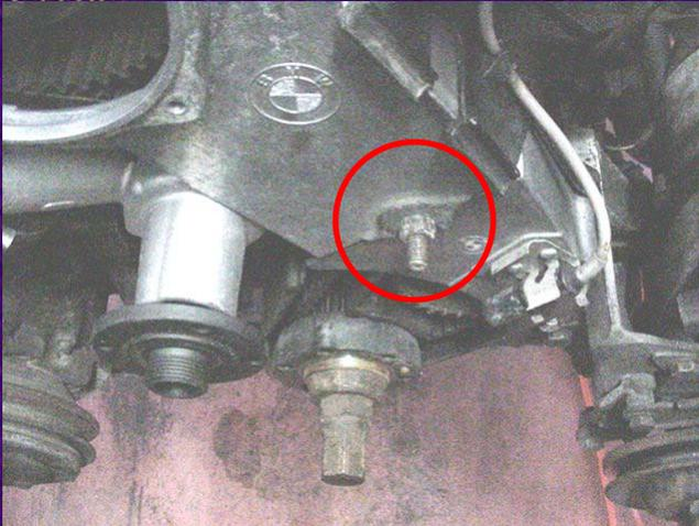
Next, install the upper timing belt cover, the black plastic protector strip and the timing sensor. Notice here that I screwed up! Attach the alternator bracket to the middle bolt BEFORE putting on the nut!
