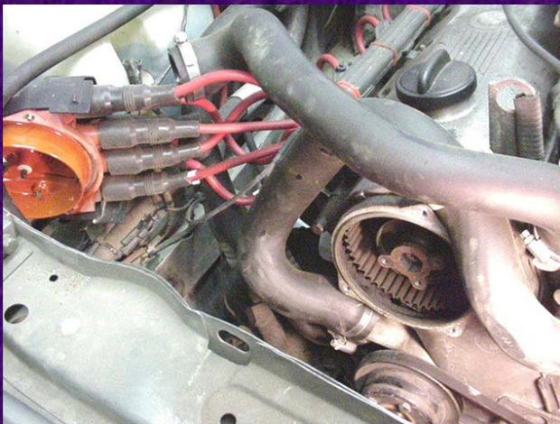
Remove the distributor cap and rotor, pushing the cap aside, with the wires still connected..
