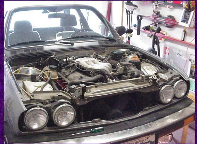
Remove the radiator by unhooking the shroud, hanging it on the fan, disconnect the top hoses and the bottom hose, and undo the two bolts and remove it
