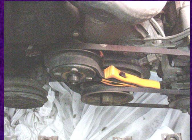
I also used the strap wrench to hold the water pump pulley while I removed its 4 retaining bolts.
