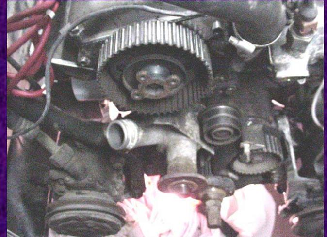
Remove the two upper bolts from the top timing belt cover, the alternator bracket, the top cover, then the lower cover bolt and cover. Loosen the top bolt on the tensioner, push it left, retighten. Snake out the belt.
