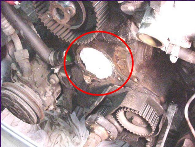
I blocked the water pump housing hole with paper towel so I could remove old gasket material and dirt from the engine without getting any inside the system.
