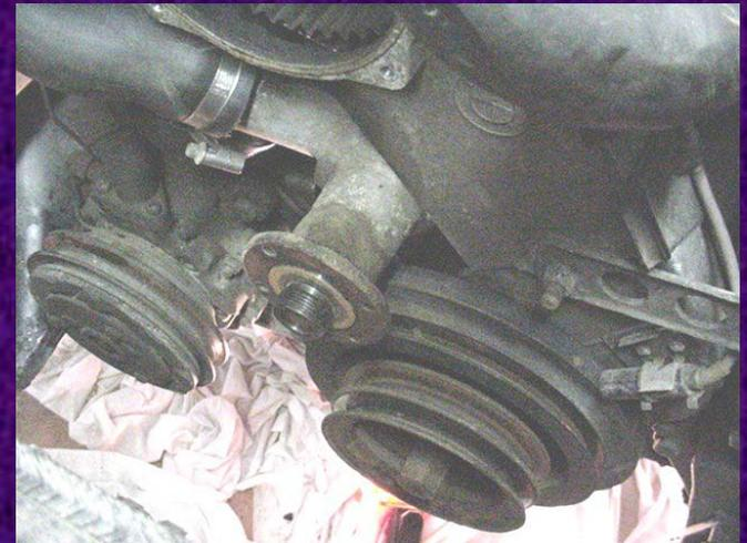
Remove the fan belts by loosening the star adjusters, slackening the alternator and steering pumps off, and removing the belts. Remove the spark plugs and rotate the engine to TDC... Leave it there and mark positions with paint!
