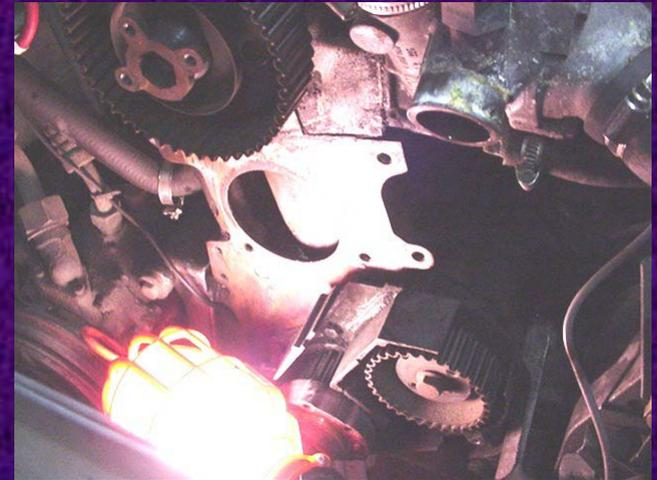
I cleaned everything, including the belt trough which was caked with grease and dirt. Once the gasket material and dirt were gone, I vacuumed all assemblies to make sure they were all dirt free. This wasn't mandatory but...
