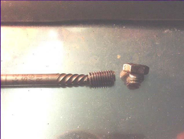
This is where I ran into trouble. I over-tightened the lower timing cover bolt and it sheared off. I was able to drill out the center of the broken bolt and removed it with an extractor.
